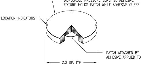
PATCH ATTACHED BY MEANS OF ADHESIVE APPLIED TO THIS SURFACE.
