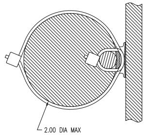
TYPICAL WIRE BUNDLE MOUNTING FOR USE WITH MS3367-1, -2, -3, -4, -5, -6, AND -7 CABLE TIE STRAPS.
