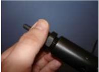
*Removing Mandrel*: Insert Mandrel adapter pin through the Mandrel release on frame head. Pull back on pin (Pull towards rear of tool). To remove mandrel, unthread mandrel by turning counter-clockwise.
