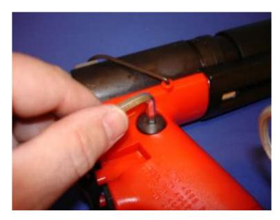
Important: Slowly poor <u>Viscosity 32</u> into bellows container provided which shall be screwed to seat on the plug. While keeping the riveting tool in a horizontal position and start air feeding, press the trigger (position 1) for the tool to carry out some cycles until air bubbles in bellows no longer come out. At this point, keep tool in horizontal position, unscrew bellows and screw 5mm hex plug back in to tool. Torque plug to minimum of 5Nm not to exceed 8Nm.
