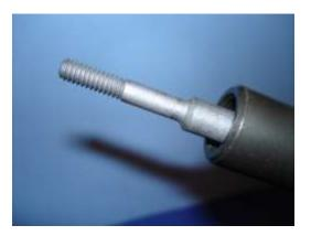
*Replacing Mandrel*: Using the same Mandrel adapter as above, pull adapter back toward rear of tool and thread new mandrel completely into mandrel housing until you hear a "Click". Thread Anvil and anvil lock nut back against frame head. Thread fastener onto mandrel, leaving .050 mandrel protruding. Unscrew anvil from frame upwards to touch the head of fastener. Tighten lock nut to frame head.
